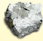
FERRO VANADIUM When added to crude steel, ferro vanadium creates a product that is lightweight and extremely high in tensile strength and wear resistance.The largest practical application of Ferro Vanadium is in the alloving process of any hardened
