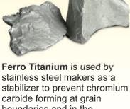
boundaries and in the production of low carbon steels for sheet production. Main applications for Ferro Titanium include: - Cleansing Agent: used for deoxidizing, desulfurization and denitrification. - Grain Refiner: improve malleability in carbon steels, thereby increasing its versatility.
