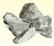
Ferro Niobium has anticorrosive properties (better than carbon steel). The adding of Ferro Niobium to an alloy can make it more weldable and much stronger. The largest practical application of Ferro Niobium is in
